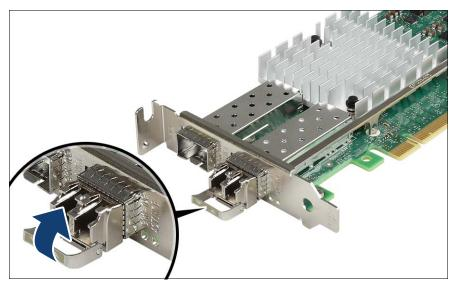
Figure 48: Latching the locking bail
